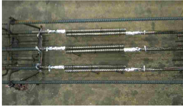
Figure 4.9 Spliced Length with Attached Strain Gauges
