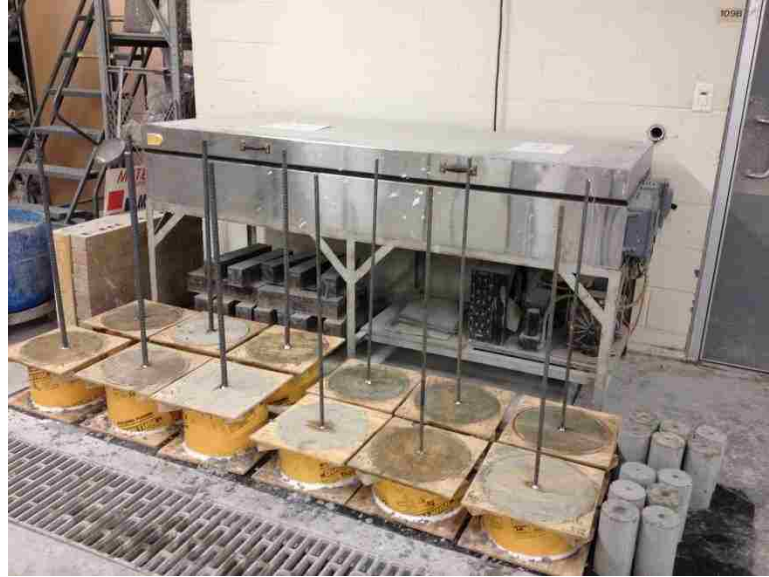
Figure 4.4 Completed Direct Pull-Out Specimens in Molds
