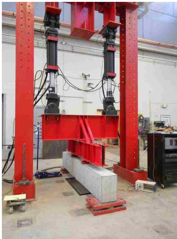
Figure 4.14 Beam Splice Specimens in Testing Load Frame
