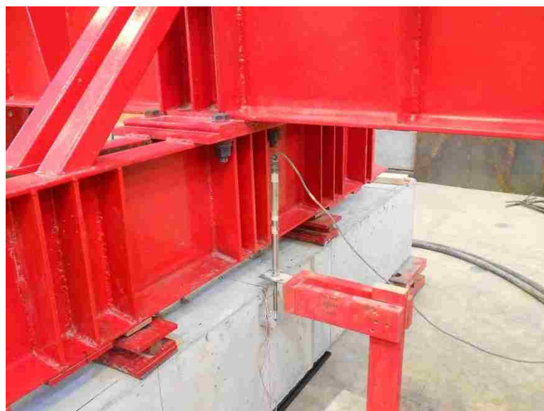
Figure 4.15 LVDT Set-Up for Beam Splice Test
