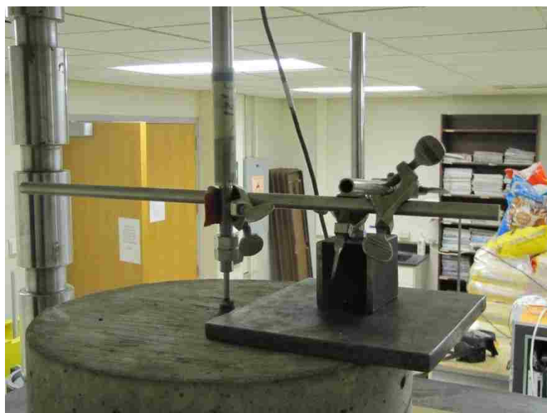
Figure 4.6 LVDT Set-Up for Direct Pull-Out Specimen
